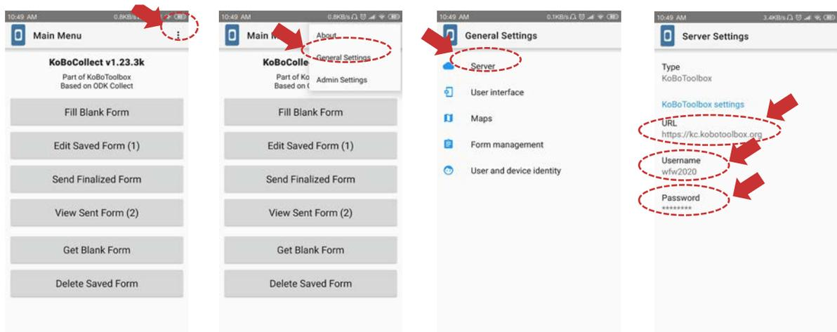
Step 1. Linking the mobile device with the Kobo account and setting up a connection to the server.
