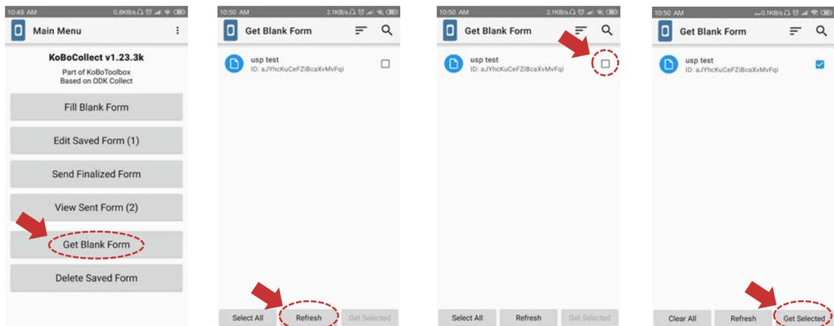
Step 2. Downloading a survey form from the Kobo account to the device.
